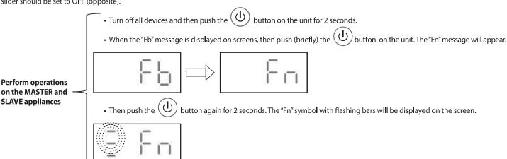
• After proper pairing, three bars will be lit simultaneously on the display of the SLAVE appliance (the bars will continue flashing on the MASTER appliance).
